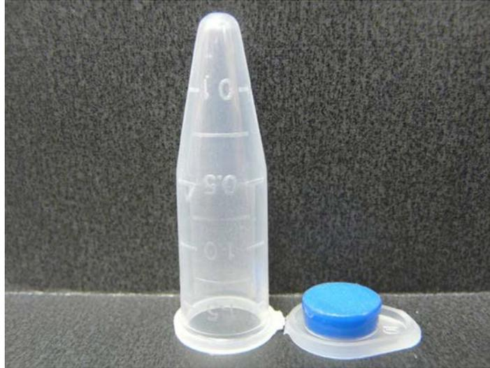
Figure 2. A 1.70 ml centrifuge tube and cap. The cap is filled with Plasticine™ to be used as a mounting medium for sectioned otoliths.
